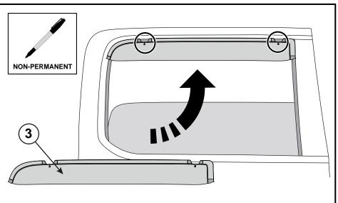
2. Pull the glass seal away from the door frame and install the clips into the seal at the noted locations.
