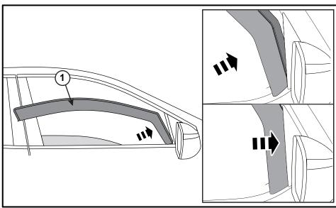
3. Fit the rear section into the door glass seal about 1/2 inch away from the top of door frame.
